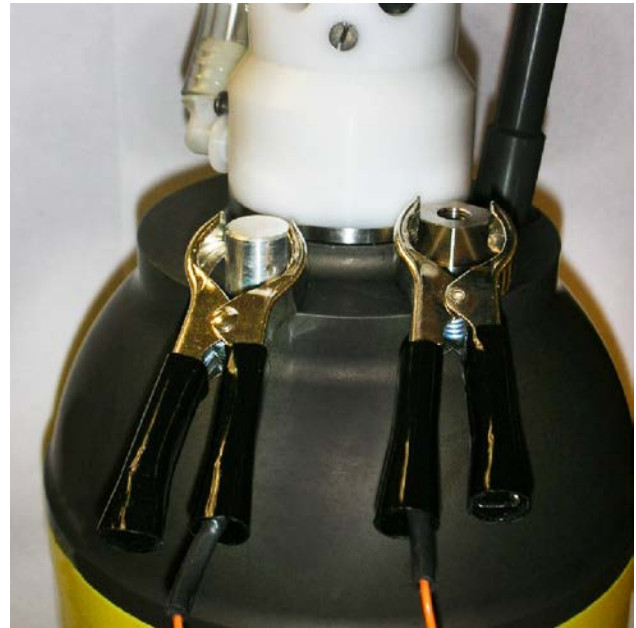
Figure 2-7: Communications Cable Connected to Zinc Anode and Terminal Post (Pressure Sensor)
